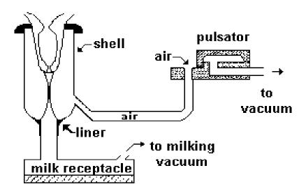
During the **milk** phase (*Figure 1B*), the space between the liner and the shell is exposed to the vacuum by way of the pulsator. The fact that there is now equal pressure on both sides of the liner causes it to open. The end of the cow's teat exposed to the vacuum and the influence of internal milk pressure within the cow's udder causes the milk to be drawn out through the teat opening.
