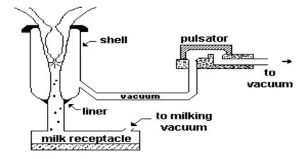
The milking process then consists of opening (milk phase) and closing (massage phase) the teat-cup liner over and over again.
