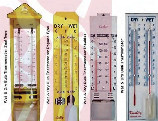
Different types of dry and wet bulb thermometers
